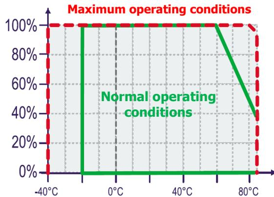
This chart shows the normal recommended operating range of the humidity sensor. Conditions outside the recommended range may temporarily offset the RH signal up to  $\pm 3\%$  RH. After return to normal conditions it will slowly return towards calibration state by itself. See "Reconditioning Procedure" to accelerate this process. Prolonged exposure to extreme conditions may accelerate ageing.
