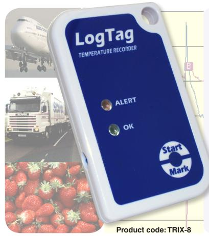
The LogTag® Temperature Recorder measures and stores up to 8000 temperature readings over a -40°C to +85°C (-40°F to +185°F) measurement range. It incorporates an external temperature sensor uniquely arranged in a recess in the case, protecting it from damage but still providing a fast reaction time more associated with remote temperature sensors.
