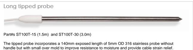
handle but with small over mold to improve resistance to moisture and provide cable strain relief. All materials at probe end of cable are FDA food rated including the cable. Supplied standard (part# ST100HT-15) with 1.5m (4'11") or 3.0m (9'10") cable terminated to MCX plug for plugging into *LogTag*<sup>®</sup> TRED30-7.
