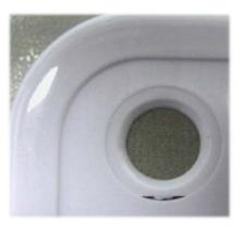
The filter is a 0.15mm thick mesh disk and is retained in the case with a specially moulded retaining ring which sits under the front label and sandwiches between the filter disk and the top label.
