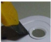
The retaining ring incorporates a cut-out section on the edge to allow prying of the ring out with a sharp knife to allow filter replacement if required.
